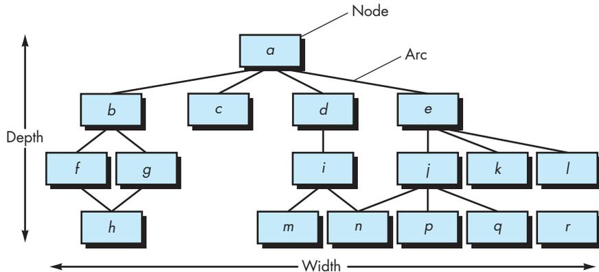
The arc-to-node ratio,  $r = a/n$ , measures the connectivity density of the architecture and may provide a simple indication of the coupling of the architecture. For the architecture shown in Figure 30.4,  $r = 18/17 = 1.06$ .
