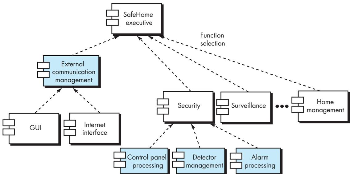
component polls sensors to detect an alarm condition, and the *alarm processing* component produces output when an alarm is detected.
