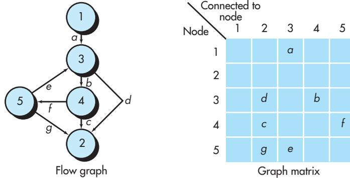
matrix can become a powerful tool for evaluating program control structure during testing. The link weight provides additional information about control flow. In its simplest form, the link weight is 1 (a connection exists) or 0 (a connection does not exist). But link weights can be assigned other, more interesting properties:
