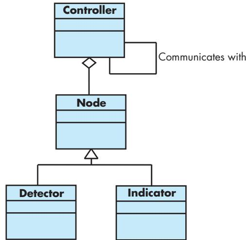
Each of these archetypes is depicted using UML notation as shown in Figure 13.7. Recall that the archetypes form the basis for the architecture but are abstractions that must be further refined as architectural design proceeds. For example, **Detector** might be refined into a class hierarchy of sensors.
