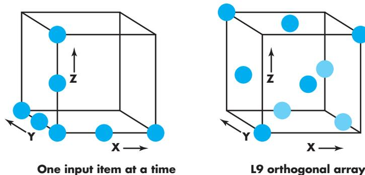
When orthogonal array testing occurs, an L9 *orthogonal array* of test cases is created. The L9 orthogonal array has a “balancing property” [Pha97]. That is, test cases (represented by dark dots in the figure) are “dispersed uniformly throughout the test domain,” as illustrated in the right-hand cube in Figure 23.9. Test coverage across the input domain is more complete.
