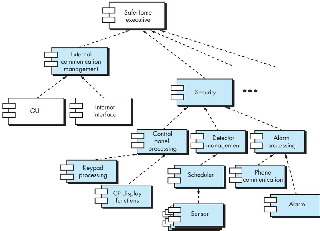
a *scheduler* infrastructure component that implements polling of each *sensor* object used by the security system. Similar elaboration is performed for each of the components represented in Figure 13.8.
