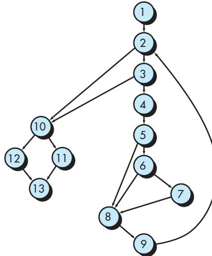
without developing a flow graph by counting all conditional statements in the PDL (for the procedure *average*, compound conditions count as two) and adding 1. Referring to Figure 23.5,
